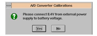
When an external power is connected, and the user selects OK to continue, the application measures a/d converter and displays the **Battery A/D Calibration** dialog box.
